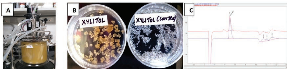
Figure 7. Showing, A, 3L lab-scale fermentor in operation with media containing synthetic xylose. B, crystallized xylitol. C, HPLC chromatogram of crystallized xylitol and control.
